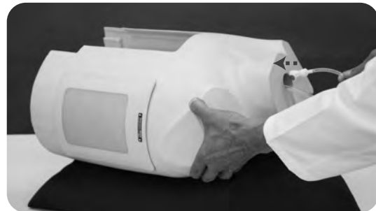
Close the cock of the three-way tap on the water drainage tube
