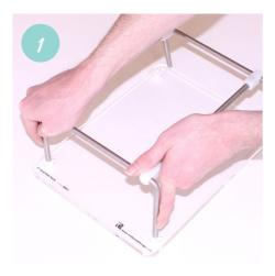
Fold down the legs of the Support Frame and insert them into the white plastic lugs as shown
