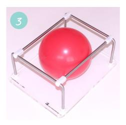
Inflate the supplied balloon and push underneath the Support Frame. Maximum diameter for the balloon should be 110mm
