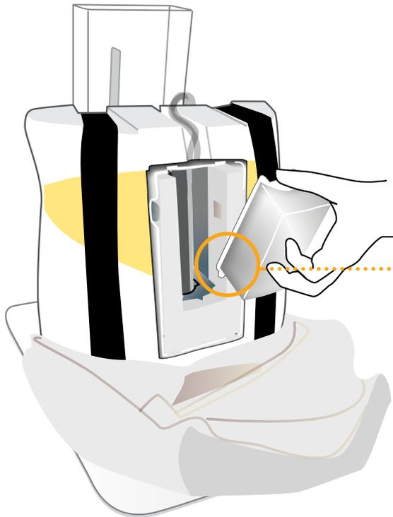
Fit lower end of insert (with teeth) first
