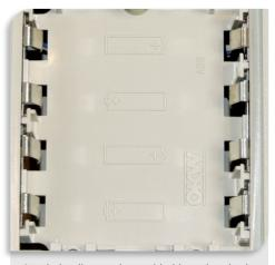
A polarity diagram is moulded into the plastic underneath the batteries.
