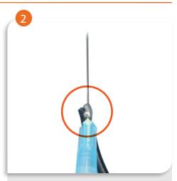
Ensure that the electrical contact is securely attached to the needle on the syringe
