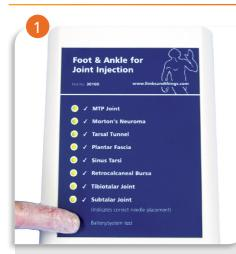
Before connecting any electrical leads, firmly press the 'Battery/system test' button on the front panel of the Feedback Console. All the lights should illuminate
