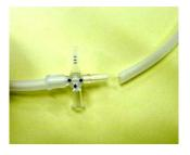
To flush the tubes quickly, it is possible to withdraw them from the three-way tap.
