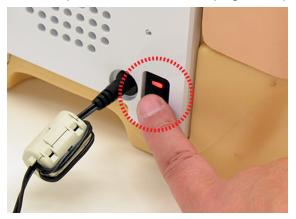
2. Unplug USB cable connecting remote controller and torso.
