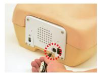
2. Connect reverse side of AC adapter to power socket.
